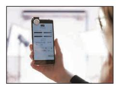
**3.** Hold your device in front of your photographic subject to measure the light. Tap the HOLD button to freeze the readings on your screen.
