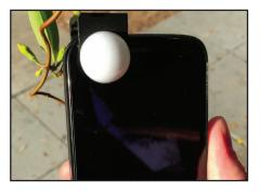
2. Attach the Luxi For All clip to your iPhone, iPad, or iPod Touch. Align the white diffusion dome so that it is positioned directly in front of the front-facing camera on your device.
